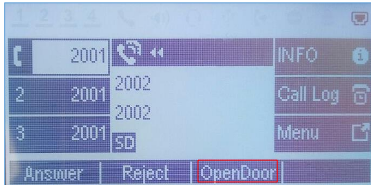
Figure 13: GDS3710 Audio Call on GXP1760 (Using SIP Server Scenario)
